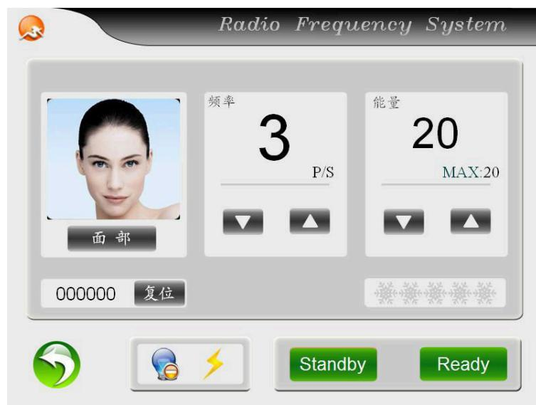
**Energy adjustment:** Click the buttons to adjust energy output of RF. The window will show the present energy value during the adjustment.
